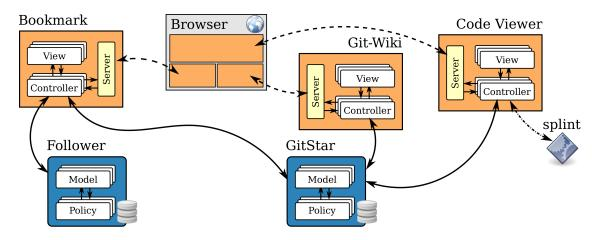
**Figure 1:** Hails platform with three VCs and two MPs. Dashed lines denote HTTP communication; solid lines denote local function calls; dashed-dotted lines denote communication with OS processes. MPs and VCs are confined at the programming language level; OS processes are jailed and only communicate with invoking VCs; the Browser is restricted to communicating with the target VCs.
